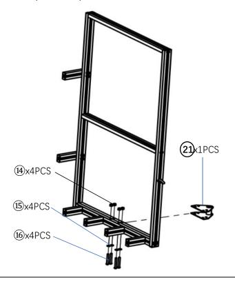
Use the hexagon socket flat round head bolt M8 \* 60 to pass through the flat washer 8x1.6 and the welding kit respectively. And tighten with lock nut M8.
