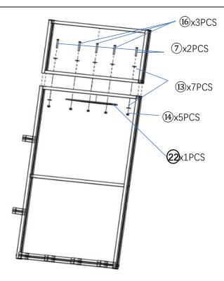
Attach the screws as shown. Pay attention to the installation direction of the outer rotating slideway.
